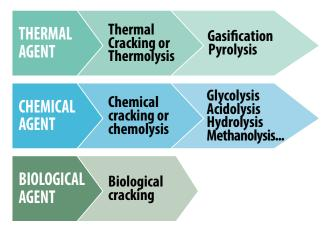
Thermal cracking (Thermolysis). The polymer chain is broken using temperature and, in some cases, catalysts. The main processes or techniques are **pyrolysis** (carried out in the absence of oxygen) and **gasification** (with oxygen). Generally, thermolysis takes place under more stringent conditions than total combustion. It is applicable to waste composed of both addition and condensation polymers.
